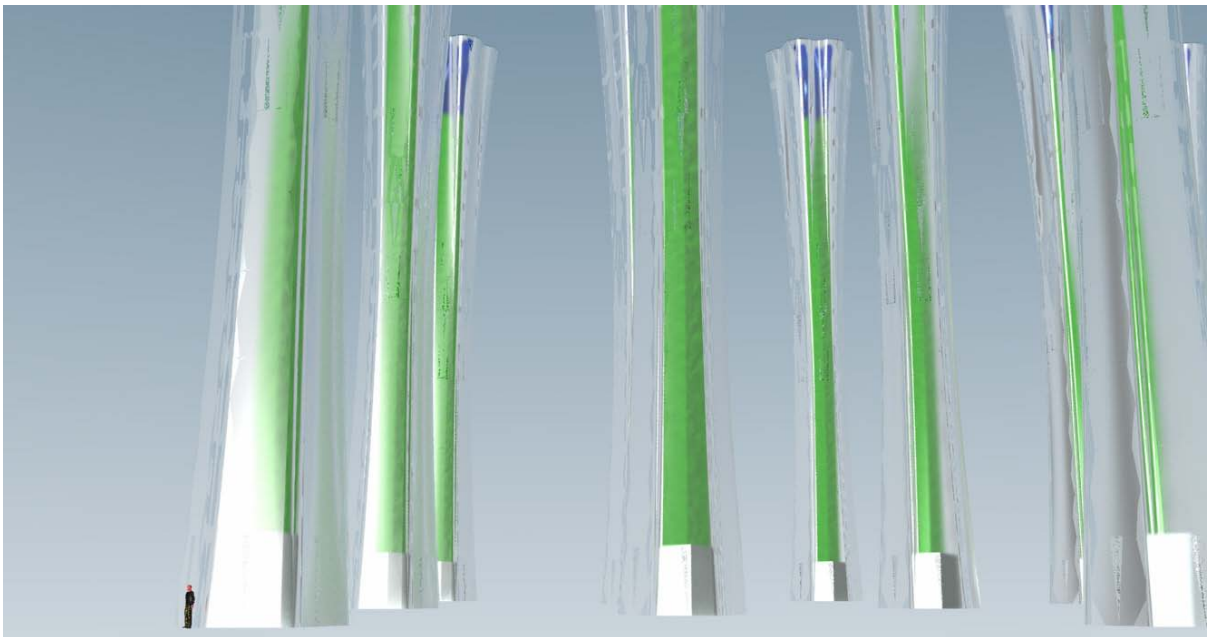
Figure 6 Biophotovoltaic masts that capture rain water to feed the algae
